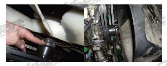
Step 10: Place a drain pan under lower radiator and heater hose connection. Remove the clamps and hoses from the radiator and allow the coolant to drain into the pan.
