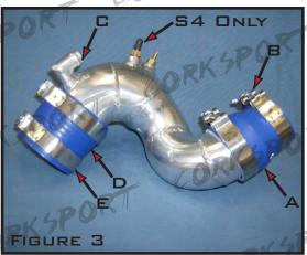
B. INSTALL 70-78MM T-BOLT BAND CLAMP ONTO THE OTHER END OF THE SILICONE CONNECTOR THAT WILL BE ATTACHING TO THE TURBOCHARGER AS SHOWN IN FIG 3, B. YOU WANT IT TO BE ALMOST TIGHT ENOUGH TO WHERE IT WON'T FALL OFF, BUT IT SHOULD NOT BE COMPRESSING THE SILICONE. THIS WILL ALLOW YOU TO EASILY GET THE SILICONE OVER THE TURBOCHARGER COMPRESSOR HOUSING INLET.
