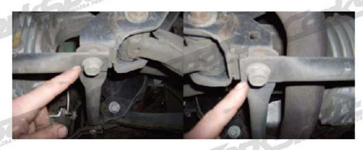
Step 5: Remove two (2) 17mm head nuts from muffler section. Remove muffler section from Miata.
