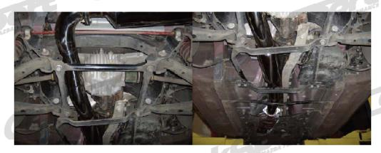
Step 12: Remove Miata from jack stands. Start up vehicle and listen for exhaust leaks. If any leaks are found recheck tightness of exhaust nuts and bolts. If no leaks found, test drive vehicle and listen for any clunking or rattling of exhaust. If there is clunking or rattling of exhaust during driving, we recommend taking Miata to your local mechanic and having engine mounts checked as well as purchasing a set of CorkSport urethane exhaust hangers
