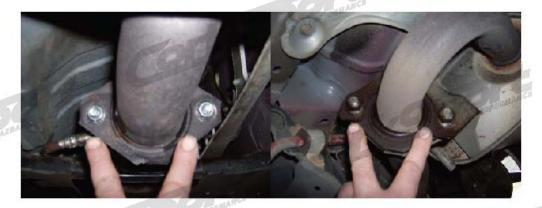
Step 3: Spray WD-40 on rubber exhaust hangers on exhaust and muffler section.
