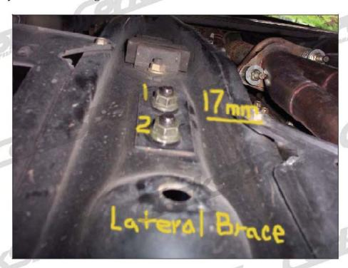
5) Replace with AWR mount or put the CS inserts in and reinstall the factory mount starting with the two (2) lower nuts. You may need to use a pry bar between the transmission case and mount to get the holes lined up for the through bolt.
