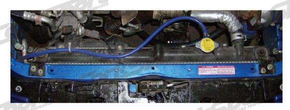
Step 2: Open your radiator cap. This is to allow the coolant to drain easier in step 4.
