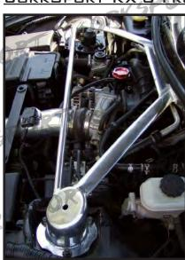
THE ONE PIECE CORKSPORT FRONT AND REAR STRUT BARS HELD INCREASE THE STIFFNESS OF THE RX-8 CHASSIS BY TYING LOAD POINTS TOGETHER. THE REDUCTION IN CHASSIS FLEX DURING HARD CORNERING RESULTS IN IMPROVED HANDLING AND STEERING RESPONSE.
